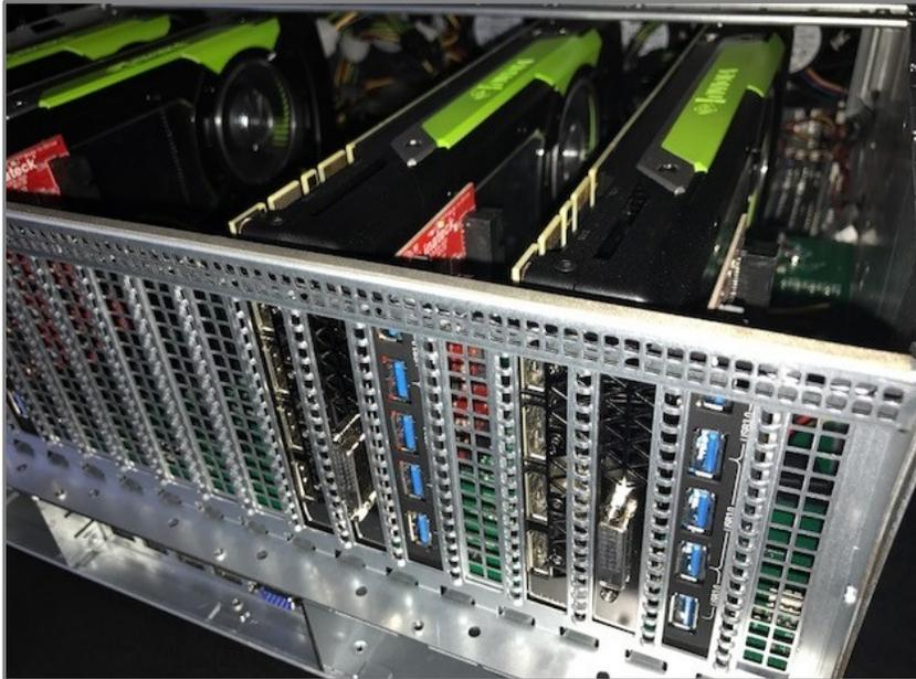
Figure 3 Quadro GPUs and Inateck USB 3.0 Controllers in the Sample System
